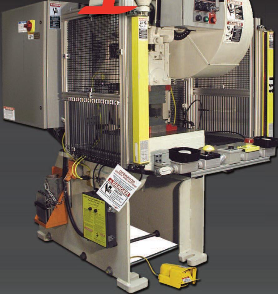
**Metalforming involves high-powered machines. Machine guards are in place to protect you from hazards on the job.**
